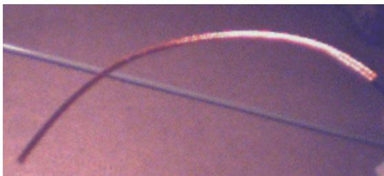
Being extremely careful not to damage the braid, I made a cut around the outer insulation of the coax at this distance and cut along it's length. This allowed me to remove the outer insulation, leaving me with the braid exposed
