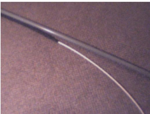
I discovered through experimentation that I actually wanted the antenna just a tiny bit short. Inserting it into it's tube had an effect like lengthening it slightly, probably due to the dielectric effect of the plastic. So the first cut you make that's too short, stop and test it in the tube... it's likely to be the exact length you need.
