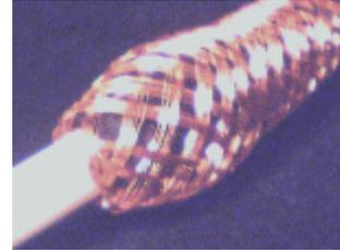
The larger picture to the left shows the antenna with the braid flipped back. At the right is a close-up of the feedpoint (where the center and braid go opposite directions) showing how the braid is flipped back over the outer insulation.
