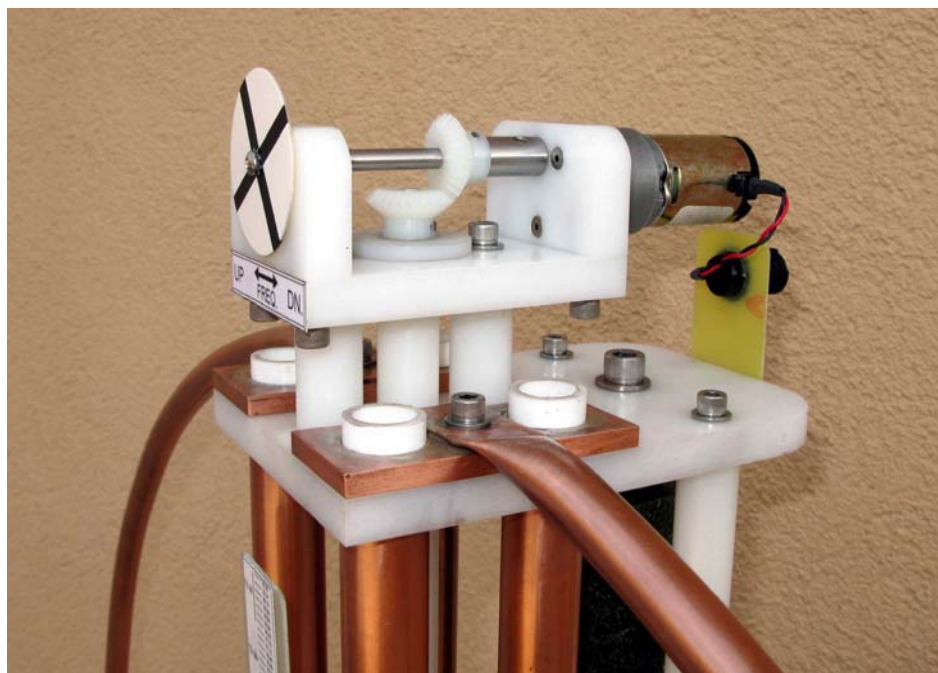
Trombone capacitor gear drive Using a www.mpja.com , #16816MD, 24 vdc, 40 rpm gearmotor
