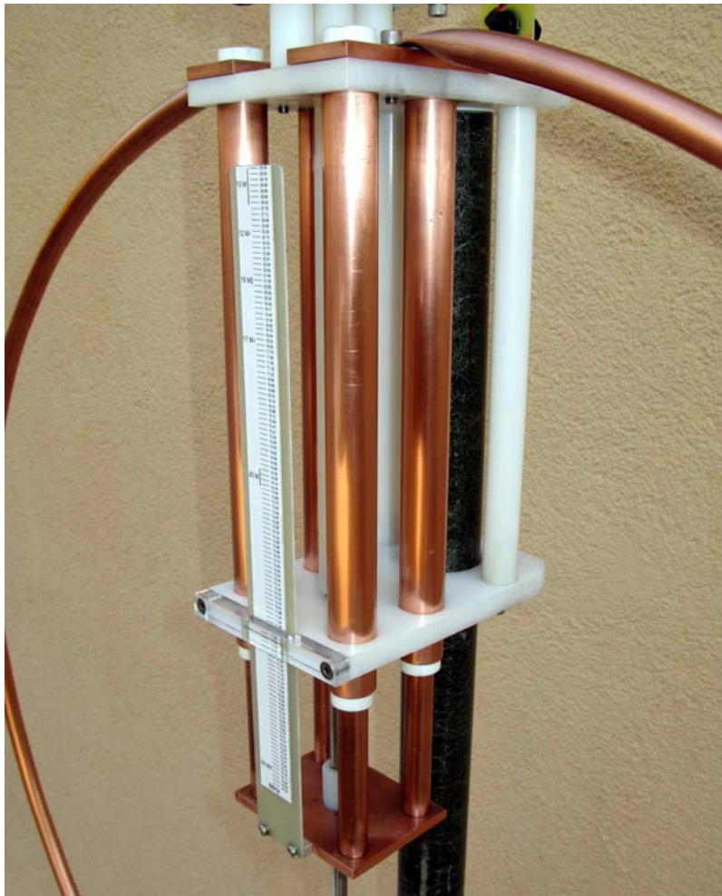
Trombone style capacitor ~10pF – ~110pF
