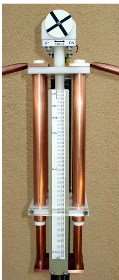
Trombone capacitor gear drive Using a www.mpja.com , #16816MD, 24 vdc, 40 rpm gearmotor
