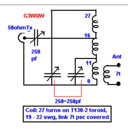
This ATU was described by **G3WQW** in Sprat 84 and being balanced can accommodate balanced line, open wire feeder or 300 ohm slotted.
