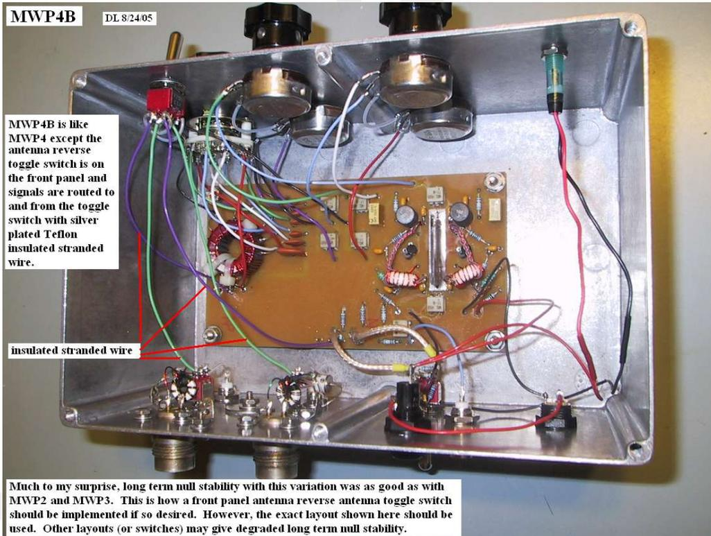
Much to my surprise, long term null stability with this variation was as good as with MWP2 and MWP3. This is how a front panel antenna reverse antenna toggle switch should be implemented if so desired. However, the exact layout shown here should be used. Other layouts (or switches) may give degraded long term null stability.
