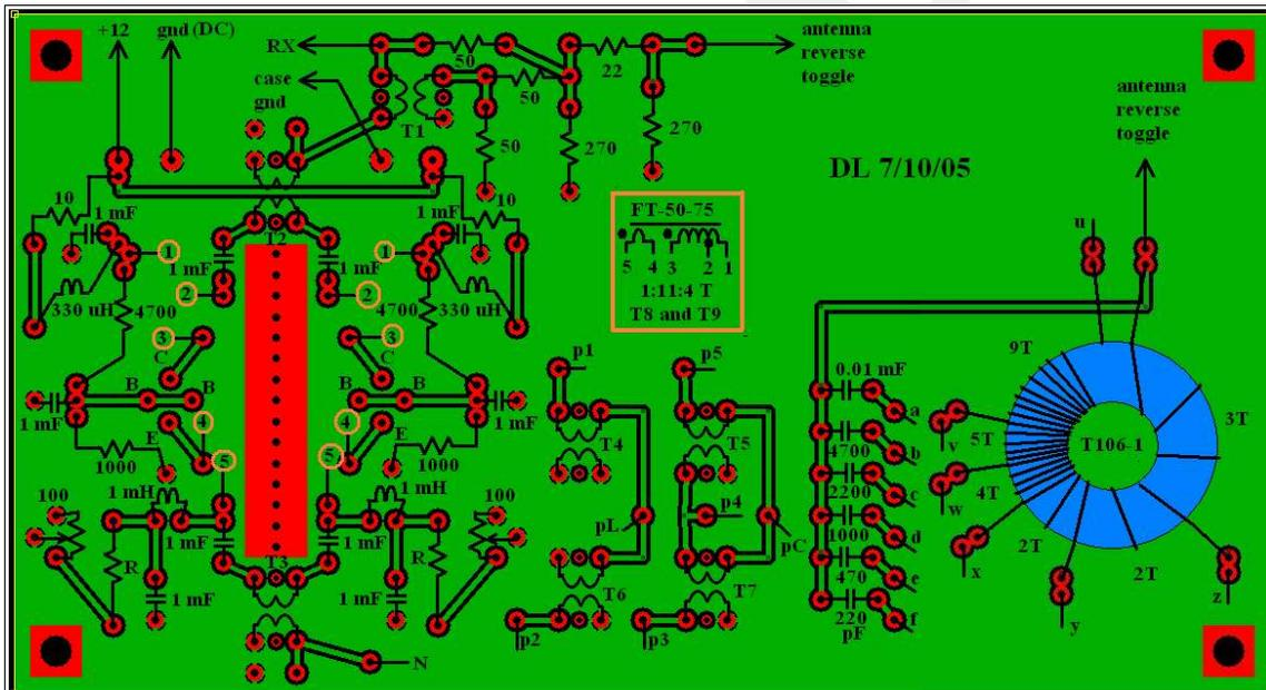
The two resistors R are 22 ohms for 2B5109's; 47 ohms for MRF581A's.
