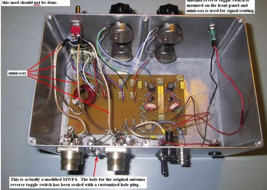
This is actually a modified MWP4. The hole for the original antenna reverse toggle switch has been sealed with a customized hole plug.
