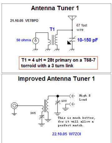
Above right: An improved version of the Antenna Tuner 1 schematic from W7ZOI. This tuner has 2 user "tweaking" adjustments much like most modern commercial antenna tuners (which typically also have a band changing adjustment). I did not build this version.
