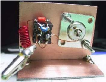
Below left: Side view, the antenna wire is held via an alligator clip. This allows me to unclip and ground the antenna when it is not in use. The antenna ground wire is soldered to the copper ground plane.
