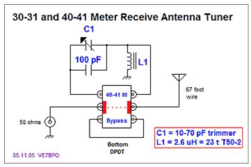
Schematic to the right: A very small receiver tuner that allowed the L network to be switched in and out of the antenna path was constructed. The L network is tuned on 40-41 meters via a small
