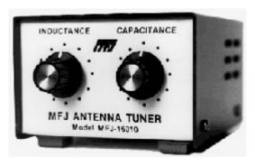
Above. MFJ web publishes their manual including the schematic for the MFJ-16010 random wire antenna tuner. The inductor is actually wound on 3 stacked (probably ferrite) cores which are tapped. The taps are connected to a front panel mounted 12 position switch. This allows coverage from 2-30 MHz. As a simple experiment, I tried stacking 2 and then 3 FT-50-61 ferrite cores and was able to get a wind range of inductances from the 6 taps I made on my test inductor.
