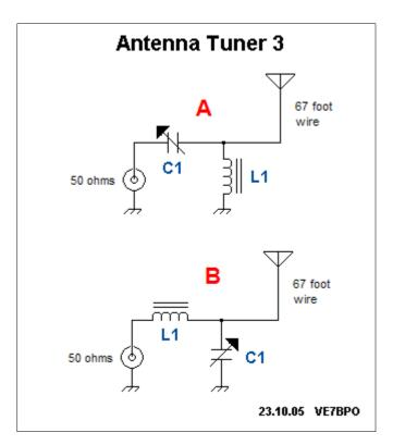
The next antenna tuner topology I tried was the familiar L network. Circuit **A** is configured in a shunt L (inductor to ground) and series C (capacitor) and is a high pass L network. Circuit **B** is configured in a series L and shunt C and is a low pass L network.
