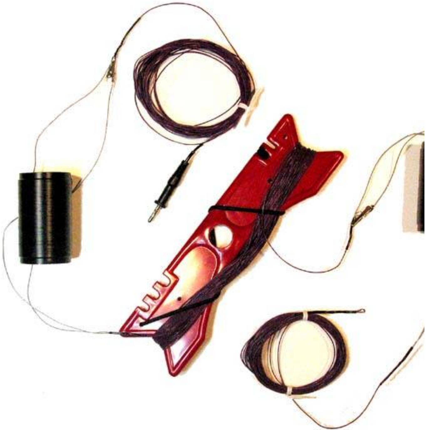
February, 2006: I built a half-sized, end fed halfwave for 160 with plans to use it during the ARRL 160 meter SSB contest. It would have been my first ever transmissions on this band. I planned to set up portable and lift the 123-foot wire with some helium balloons and operate in the QRP category. Long story short is that I drove 50 miles round trip to buy two
