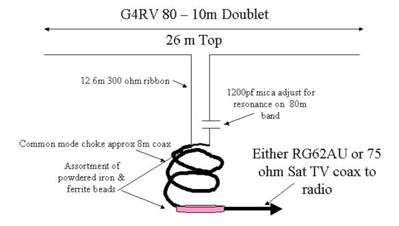
Antenna resonant on 40, 20, 10m ATU required on other bands
