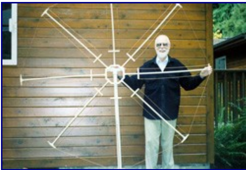
The completed 15 meter convoluted full-wave loop antenna, with the author.
