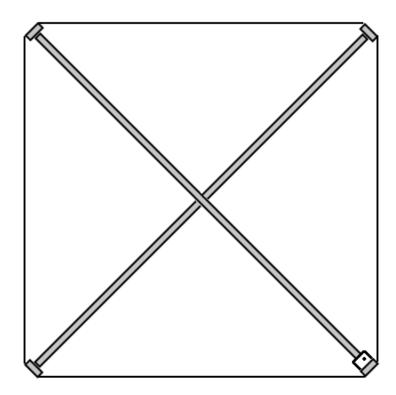
• At the end of 9 turns, route the other end free end of the wire through the end hole in the tuning block, and attach to the primary screw on the terminal block.
