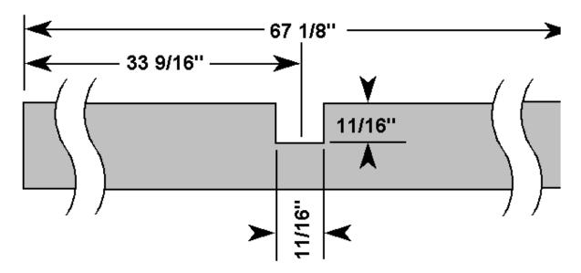
Make an "X" from the two braces by fastening them together at the notches. Make sure the boards fit together flush, and the two braces form a 90 degree angle. They can be secured with wood glue, or with a screw if the loop must be disassembled.
