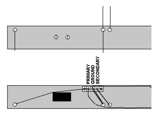
Connect the ground terminal screw on the terminal block to the ground of the receiver. Connect the secondary screw on the terminal block to the antenna input of the receiver. Use coax or twisted pair to connect to the receiver.
