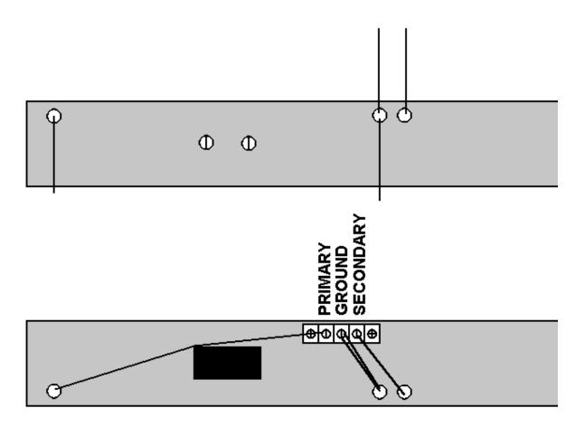
Connect the ground of the tuning capacitor to the ground screw of the terminal block. Connect the other terminal of the tuning capacitor to the primary screw of the terminal block.
