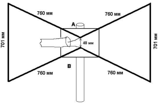
The antenna is made from a copper or aluminum wire in diameter of 4 mm. A copper or brass tube also will do well. The wires fastened by collars to a dielectric plate in 4 mm thickness. I use a plate from PC stuff. The plate fastened by collars to the antenna metal mast.
