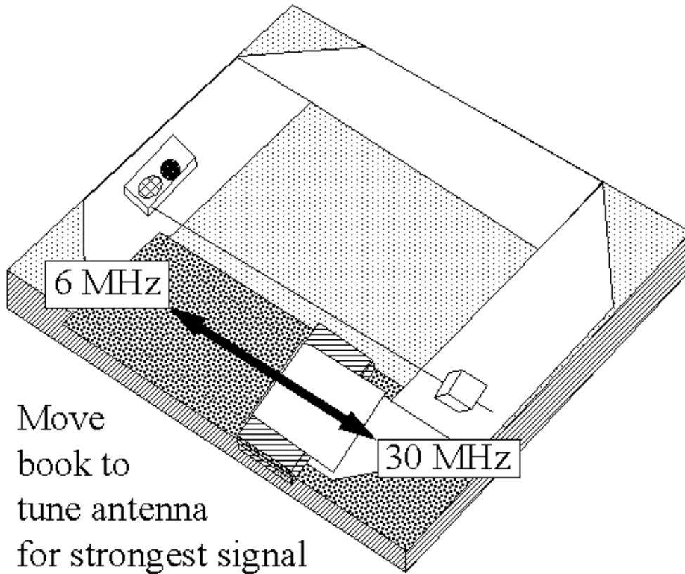
If you use a table model receiver (or an amateur transceiver,) make a single turn loop of about #18 insulated hookup wire by taping the wire in place one inch inside the foil loop. Bring the wire away from the antenna on the middle of the side opposite the tuner. Don't connect this loop to the foil - it isn't necessary.
