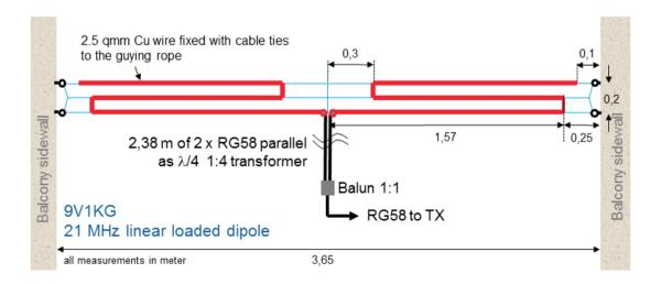
First measurements at the resonance frequency showed a low input impedance at the dipole's feed point with values around 10 Ohm. The theoretical radiation resistance of a 2 x 1.6 m short dipole would be 10 Ohm, so it is an indication of low losses in the system. In order to match the antenna to the 50 Ohm of the transceiver, I use a quarter wave transmission line transformer consisting of two parallel connected 50 Ohm coaxial cables.
