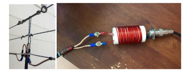
Dipole feed point and 1:1 balun Posted on2016-03-30AuthorKlausCategories9V1KG, Amateur RadioTags9V1KG, antenna, balcony, linear loaded, short dipole
