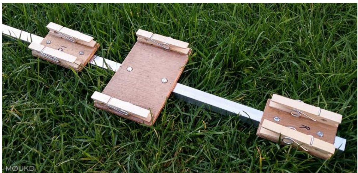
The driven element has a larger plate to accommodate the box which contains the choke and driver assembly.
