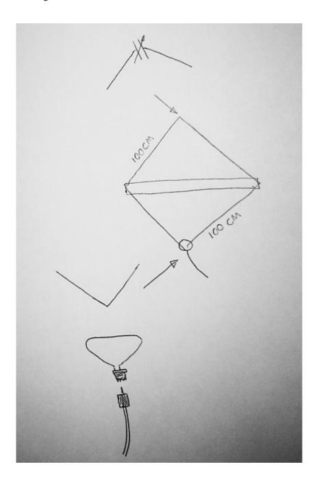
At the bottom a simple pick up loop is taped to the main loop. No direct electrical connection is made to the main loop.
