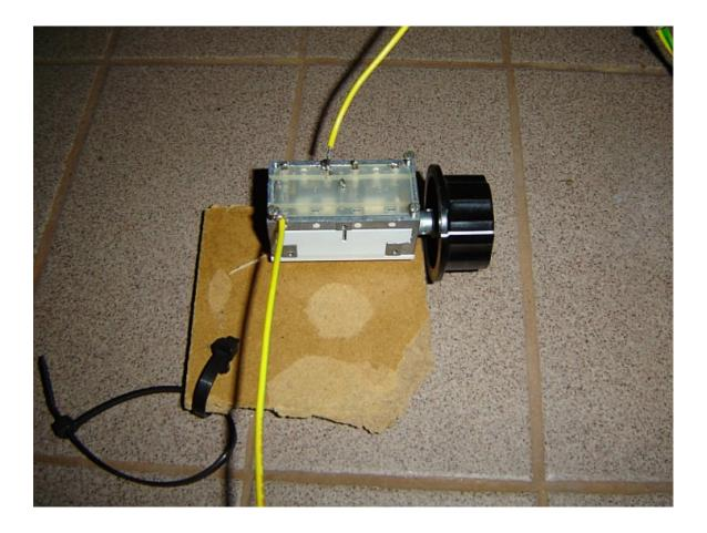
In operation the loop shows a deep null off to the side, just the thing to knock out a strong SW or undesirable stations on the frequency you want to listen on.
