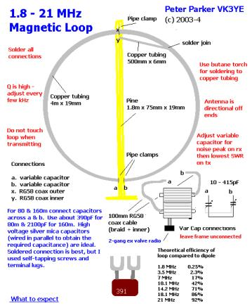
Magnetic loops are a compromise antenna and performance will be down on a full-size wire antenna, particularly on the lower HF bands. If built properly, expect the following results at QRP power levels: (i) 80 metres - contacts up to a few hundred kilometres, (ii) 40 & 30 metres - single hup contacts up to about 1000 km, (iii) 20 metres - contacts up to about 3000 kilometres with the occasional DX. The variable capacitor won't spark if transmit power is kept down (10w is fine).
