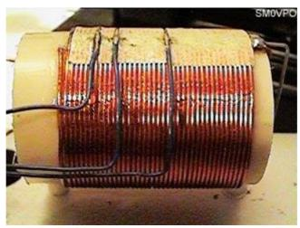
With this switchable coil you will be able to match a random length wire antenna over most of the HF band. The tuning procedure is exactly as given above but select the switch position that gives you the best match.
