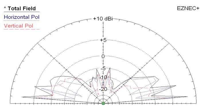
3 Turn stretched helix fed with gamma match at centre at 10m above ground with coax
