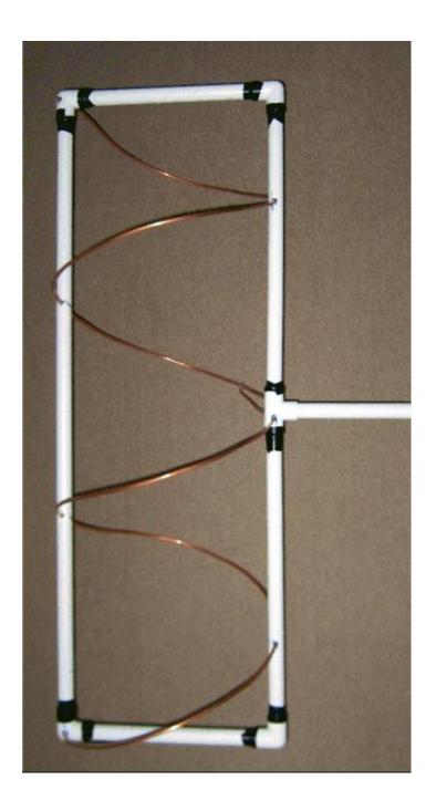
The turns of copper pipe are held in place by a single turn of thin copper wire wrapped around the pipe and soldered close to the plastic pipe. The antenna is quite high Q so requires some fine tuning once built. I made the last turns slightly longer than required and then cut them to resonance. Painting the antenna will lower the resonant frequency slightly. Very fine tuning can be achieved by bending the gamma match wire.
