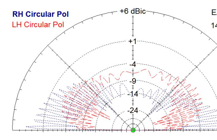
Pattern is Omni-directional with very slight asymmetry due to the gamma match and interaction with the mast and feed coax.
