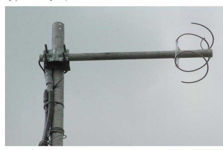
Andy has reversed the direction of the feed coax so that it passes through the center of the helix.
