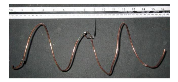
Fixed the antenna to a short length of plastic tube in the workshop, and checked with a hand held fluorescent tube to see if the voltage distribution looked even between turns. Got the lamp to strike and then wound the power down to about 5 watts so that I could see the areas of the tube that remained lit up more clearly. Observed four distinctive bright spots of similar luminance (although it's not that clear in the photo) at each of the high voltage points.
