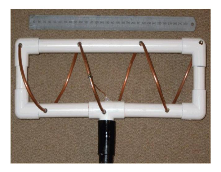
The turns of copper pipe are held in place by a single turn of thin copper wire wrapped around the pipe and soldered close to the plastic pipe. The antenna is quite high Q so requires some fine tuning once built. I made the last turns slightly longer than required and then cut them to resonance. Painting the antenna will lower the resonant frequency slightly. Very fine tuning can be achieved by bending the gamma match wire.
