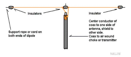
It consists of 2 equal lengths of #12 or #14 wire insulated in the center and on each end and supported with rope, nylon cord, etc from both ends and the center if needed.
