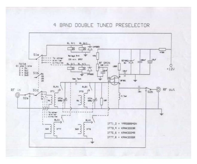
The circuit requires an RF input which can be from a longwire or a loop antenna. The Preamplifier has a range from 550kHz (Medium Wave) up to 30 MHz in the SW band. The input Switch S1, applies voltage to a set of relays which switch in the appropriate coils.
