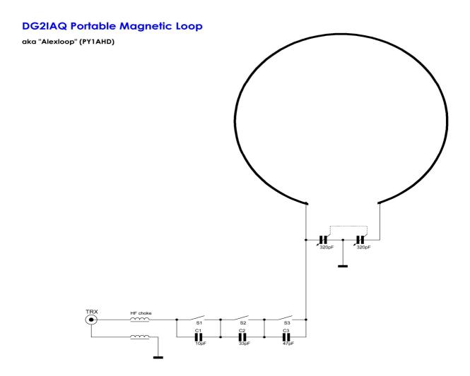
The basic idea was to improve the great design of the portable "Alexloop" of PY1AHD by removing the coupling ring and replacing it by a low-loss capacitance matching unit.
