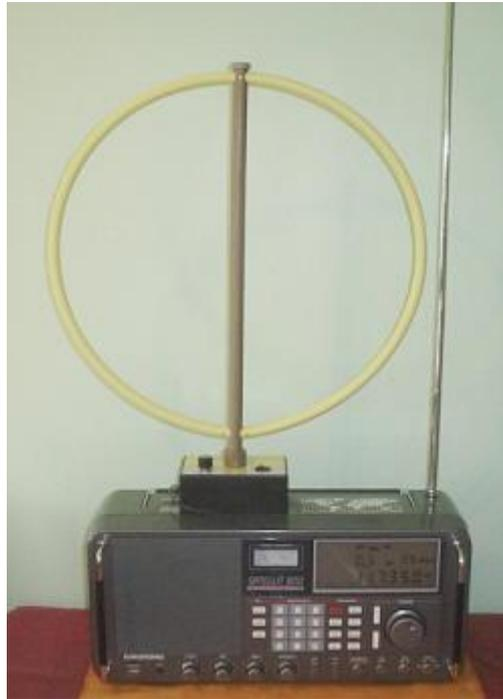
**Antena Loop Coaxial Magnética**
