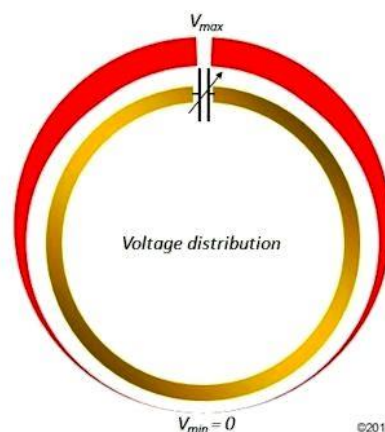
Fig. 3: Voltage distribution around a loop antenna
