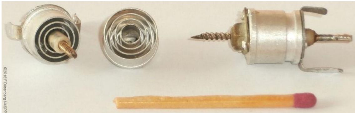
Fig. 13: Philips tubular-piston trimmer capacitors (5-30 pF, 0.3 mm plate distance)
