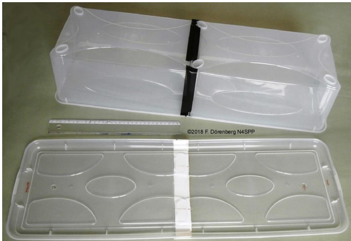
Fig. 122: Protective hood made of two clear plastic boxes and their lids
