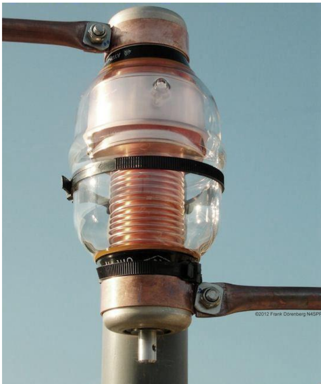
Fig. 79: My vacuum capacitor, attached to the mast and connected to the loop
