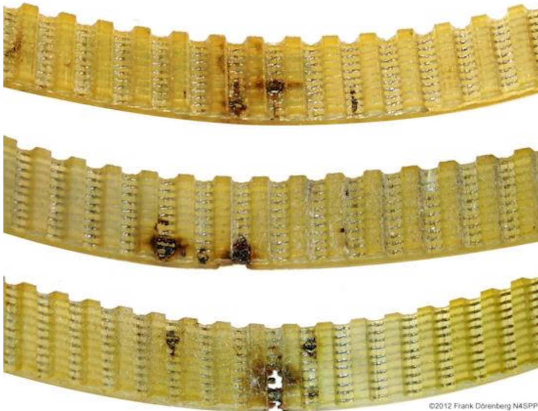
Fig. 101: Arcing damage to the steel-reinforced belt
