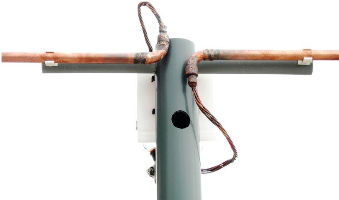
Fig. 48: The back side of the capacitor mounting (the hole in the mast is for inserting a socket wrench for tightening the nut on the bottom bolt of the capacitor mounting board)
