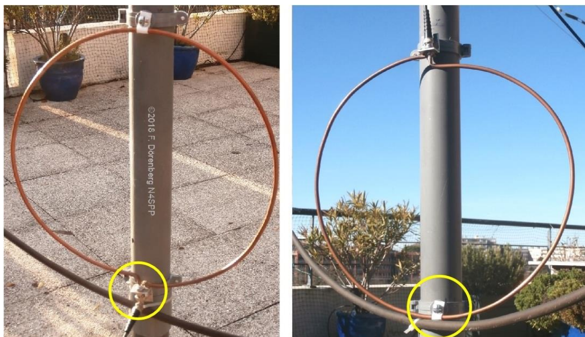
Fig. 84: The two configurations of my coupling loop (the BNC connector is mounted on a small aluminium L-bracket)
