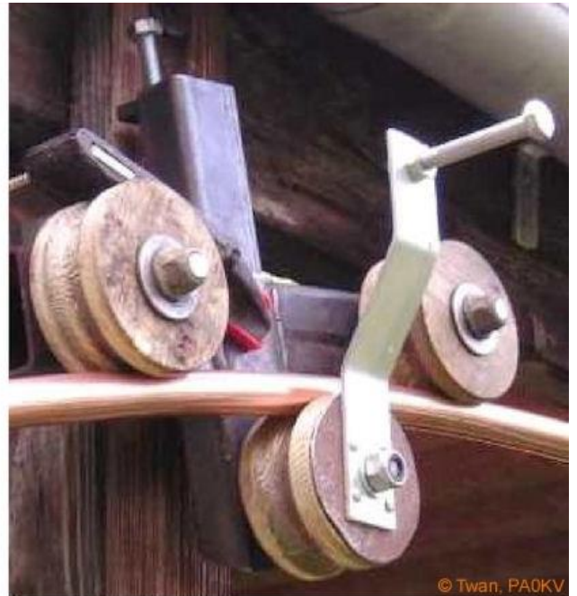
Fig. 76: A sturdy tube bender made by Twan van Gestel (PA0KV) (photos used with permission; his large loop with motorized vacuum capacitor is described on his website [pdf] )
