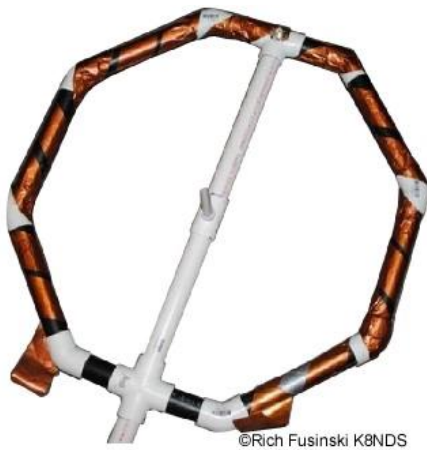
Fig. 9: Flat conductor loop (helically wound/loaded, shown without capacitor) and Slinky™ coil loop (sources: ref. 5A/B and 5C)
