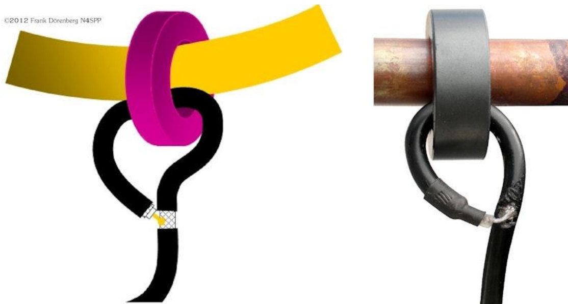
Fig. 26: A 1:1 ferrite transformer-coupling with coax loop as secondary winding
