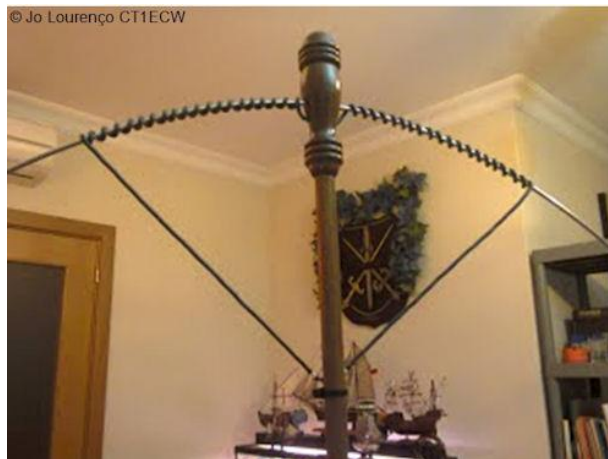
Fig. 20: Spiral coupling (photo: ©Jo Lourenço, used with permission)
