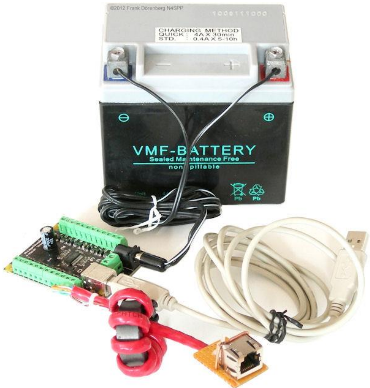
Fig. 103: Toroidal current choke on the CAT5 cable between controller card and stepper-motor
