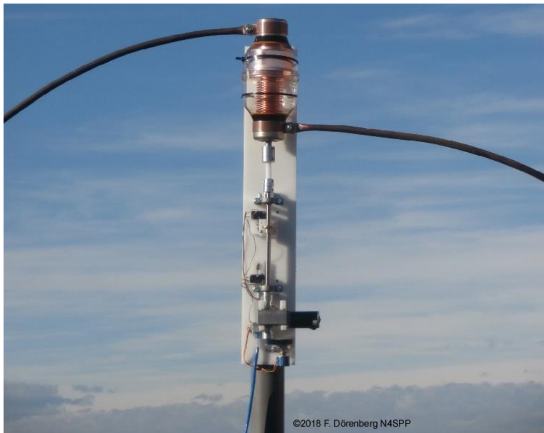
Fig. 121: Motor drive installed on the PVC-tube antenna mast
