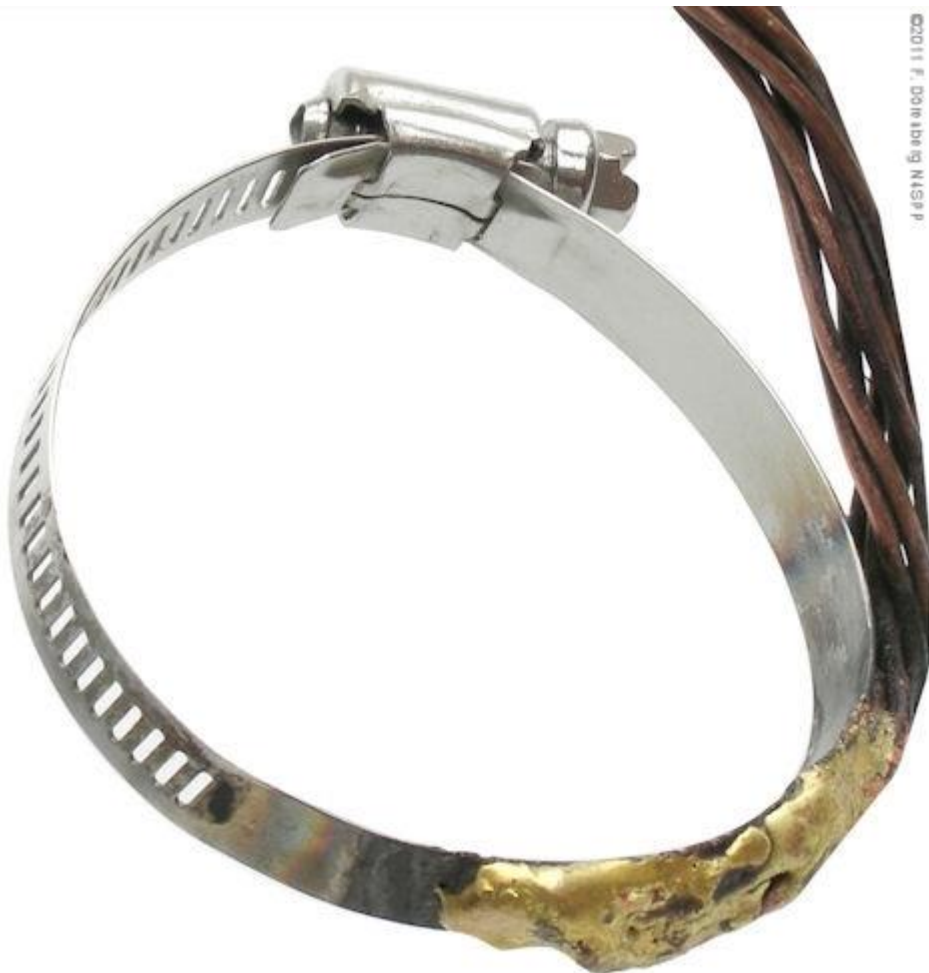
Fig. 49: Close-up of the capacitor connection wire, brazed to a copper reduction piece on the loop-ends
