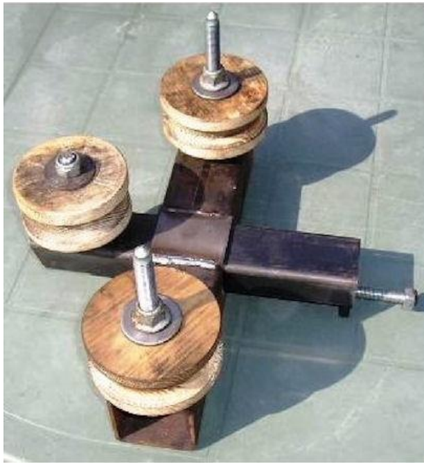
Fig. 76: A sturdy tube bender made by Twan van Gestel (PA0KV) (photos used with permission; his large loop with motorized vacuum capacitor is described on his website [pdf] )
