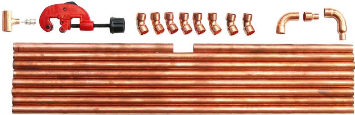
Fig. 41: The "plumbing" parts of my STL antenna (tubing, elbow pieces, T-piece) and a cutting tool
