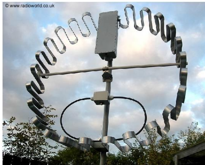
Fig.10: Flat conductor loop and meandering "fractal" loop (source: ref. 4 and www.radioworld.co.uk )
