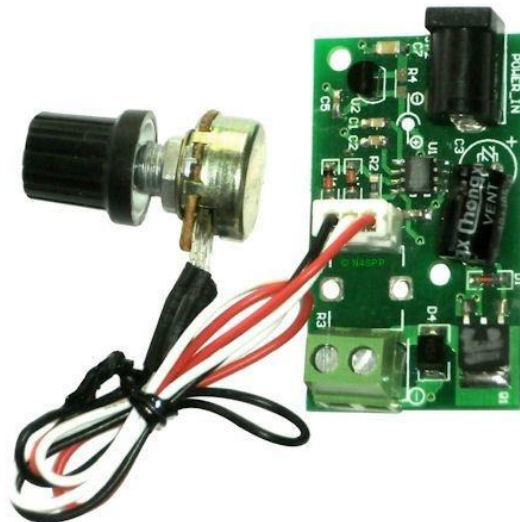
Fig. 126: The small PWM speed controller card
