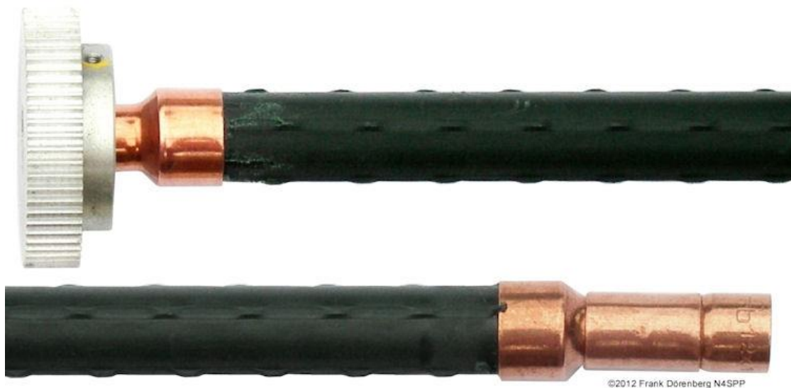
Fig. 106: Plastic drive-shaft with gear wheel installed
