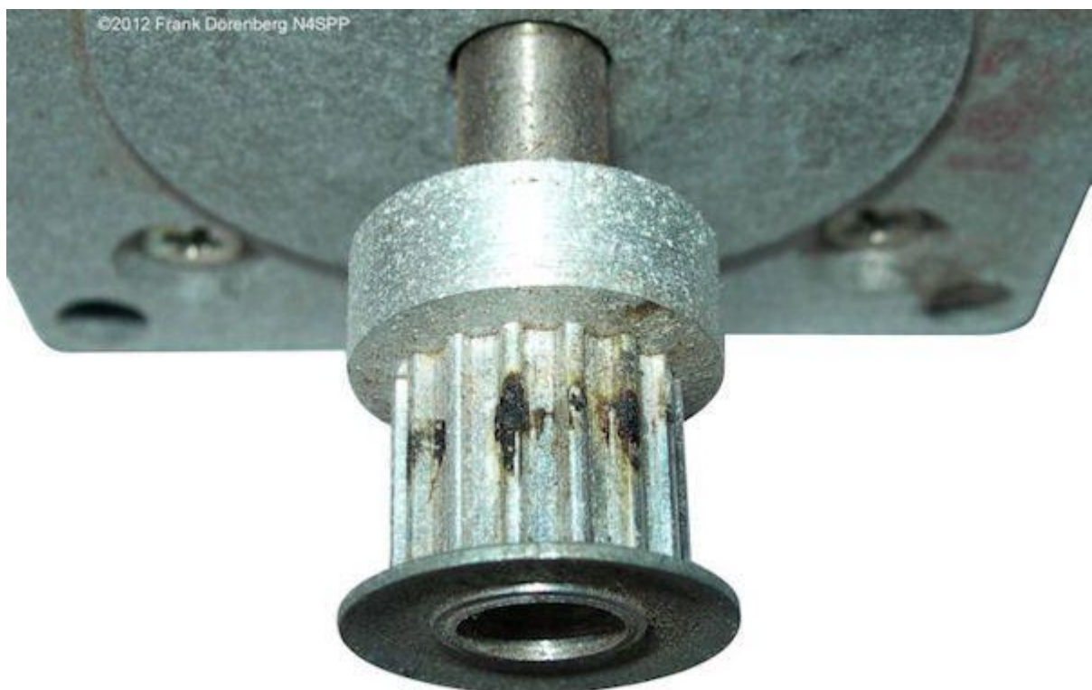
Fig. 102: Arcing damage to the pulley of the stepper-motor
