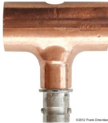
Fig. 34: Copper T-piece - inserted into the main loop at the neutral point - with BNC connector
