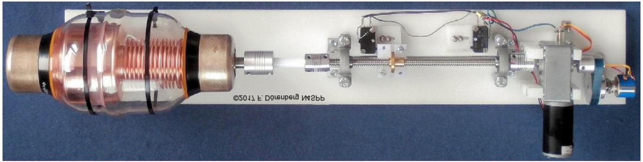
Fig. 114: Top view of the DC motor drive assembly with vacuum capacitor
