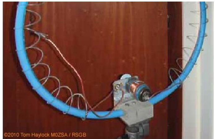
Fig. 9: Flat conductor loop (helically wound/loaded, shown without capacitor) and Slinky™ coil loop (sources: ref. 5A/B and 5C)
