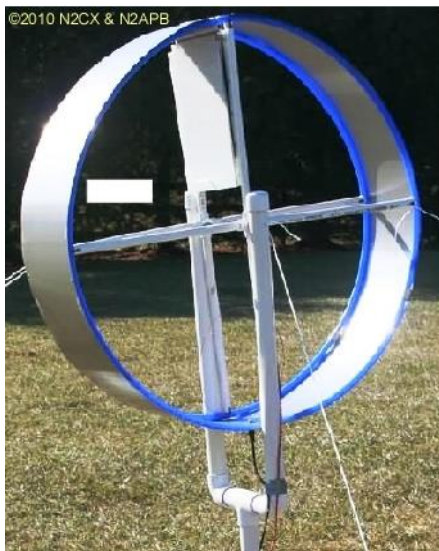
Fig.10: Flat conductor loop and meandering "fractal" loop (source: ref. 4 and www.radioworld.co.uk )
