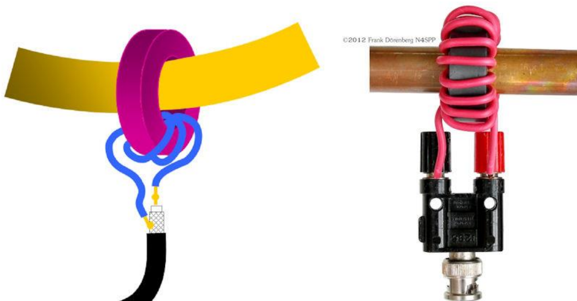
Fig. 27: A 1:N transformer coupling with a ferrite core
