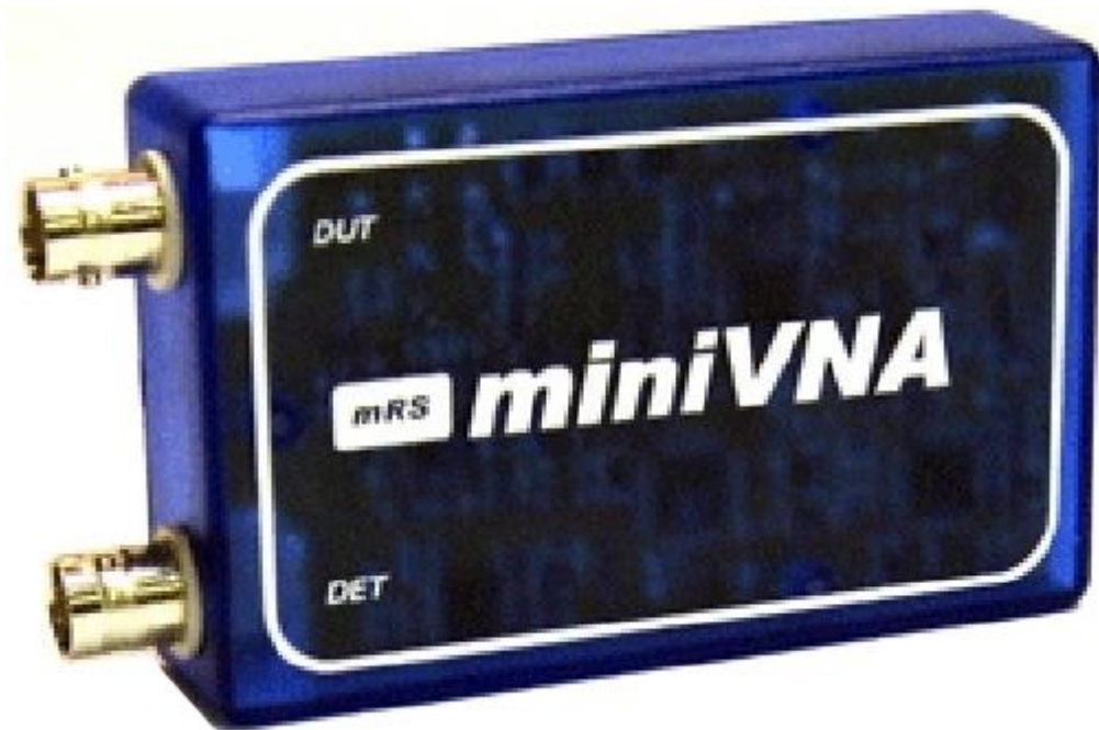
Fig. 64: My miniVNA - a tiny antenna analyzer for 0.1-180 MHz, with USB connection to a PC
