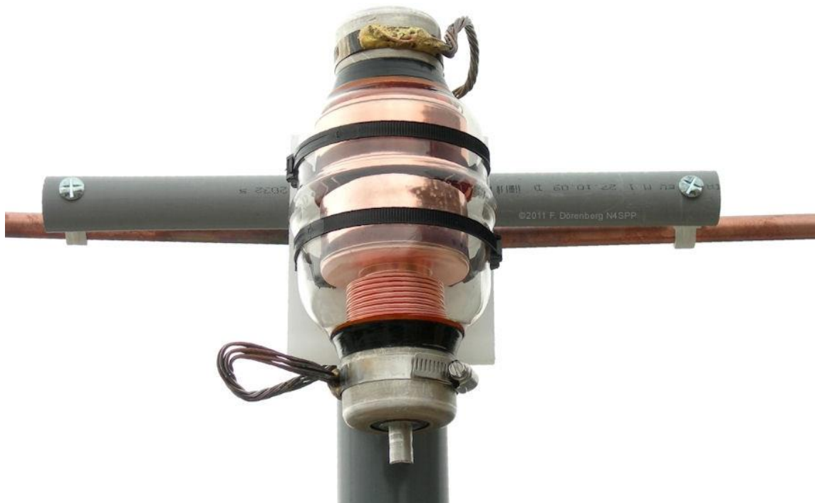
Fig. 61: The vacuum capacitor mounted at the top of the mast
