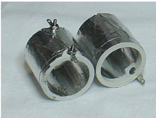
Photo A: Home-built Trap Capacitors
