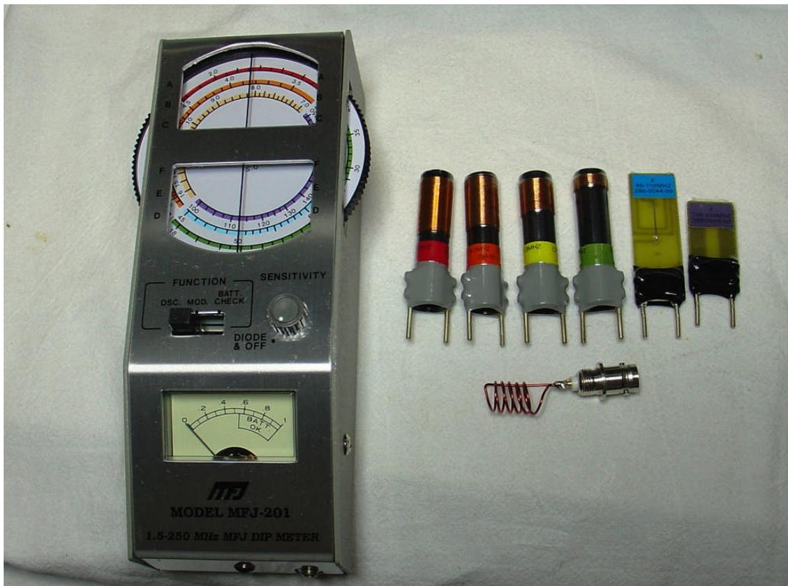
Photo D: The MFJ-201 Grid-Dip Oscillator
