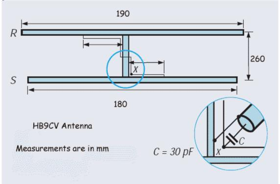
The boom is 25x25 mm made of aluminum. Elements are 1mm round aluminum. The 15 pf capacitor (fixed) is mounted at the front of the antenna. See photo for mounting detail. However, you may want to use a small 30pf variable to get the SWR as low as possible then replace it with a fixed value. A 15pf will work fine if you have no way to check the final capacitance. I suggest you extend the boom to hold onto it and perhaps mount your portable 2m radio on it somehow. Good fox hunting. VE3COJ
