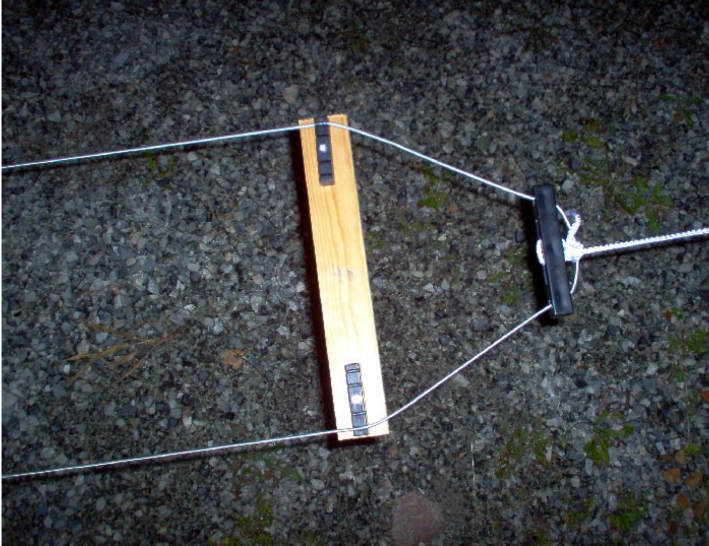
The end isolator and the spreader. The spreader are made out of wood, with plastic isolators mounted on.
