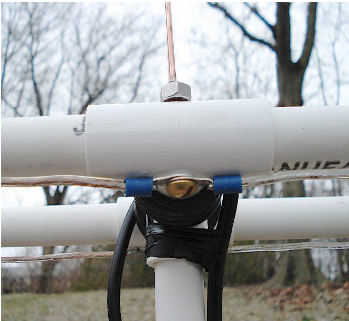
Photo of rear "center" element on reflector portion of antenna. Notice connections to each outside element using speaker wire.
