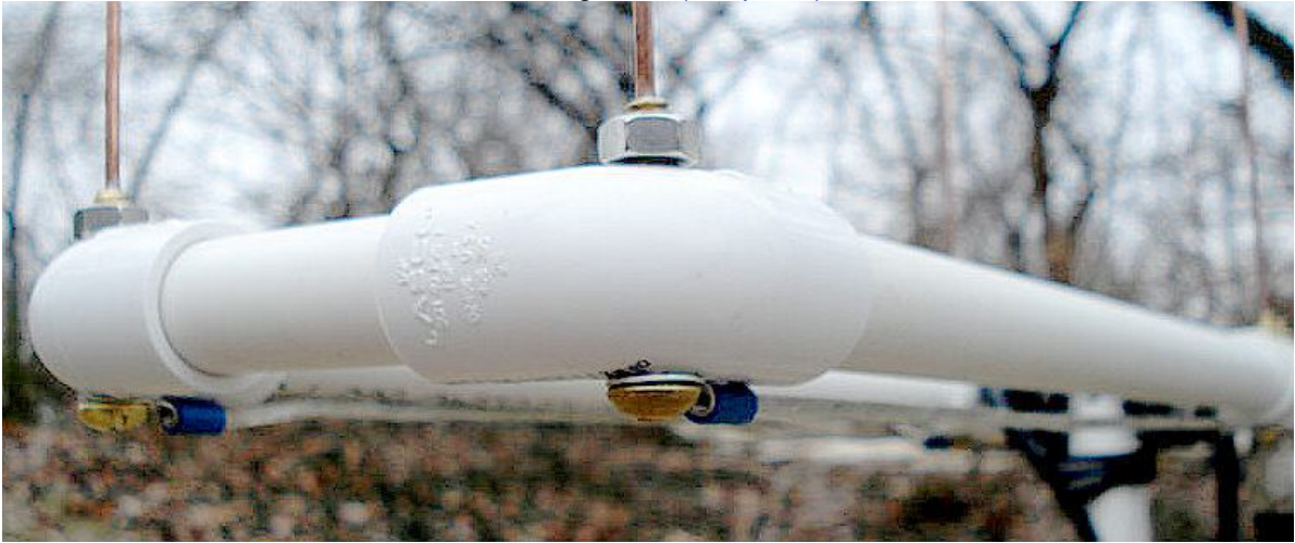
Photo showing ends with elements, ring lugs and wire extending from them.
