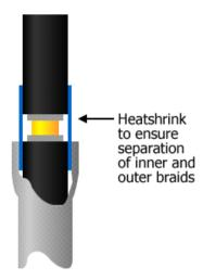
Piece of heatshrink acting as a separator at the radiator feedpoint
