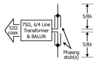
The double 5/8 is a co-axially fed variation of the 11/4 wave (vertical) dipole
