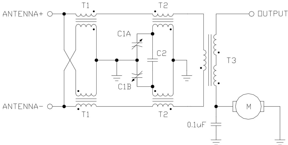
Fig. 6 - Transmitting Loop Antenna Tuner Schematic
