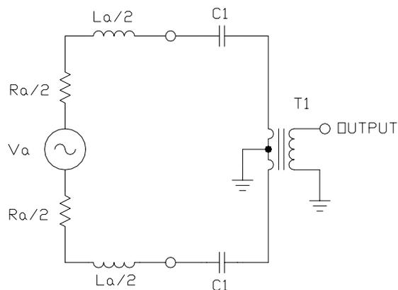
Fig. 3 - Basic Passive Series Tuning
