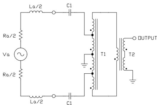
Fig. 4 - Passive Series Tuning with 1:4 Transformers
