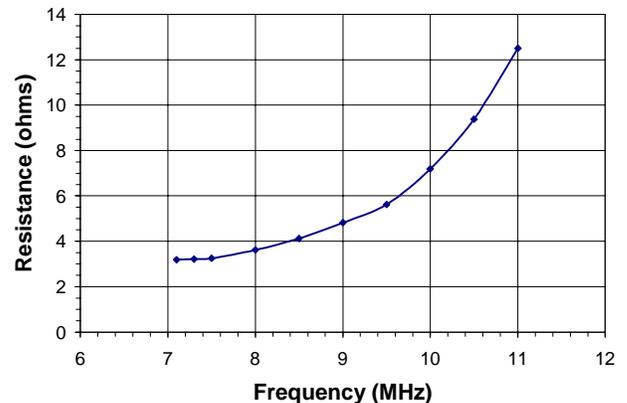
Fig. 1 - Measured Resistance of 1.5 meter Diameter Loop Antenna made with 1/2" Copper Tubing
