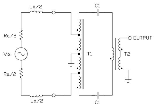
Fig. 5 - Passive Series Tuning with Relocated Series Capacitors
