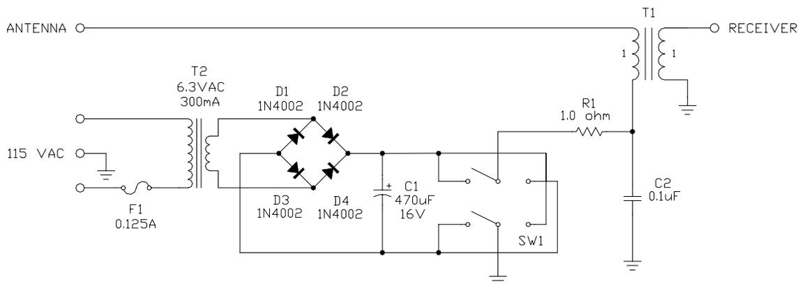
Fig. 16 - Simple Control Unit Schematic (see text)
