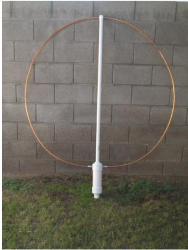
Fig. 15 - Completed Transmitting Loop Antenna Assembly
