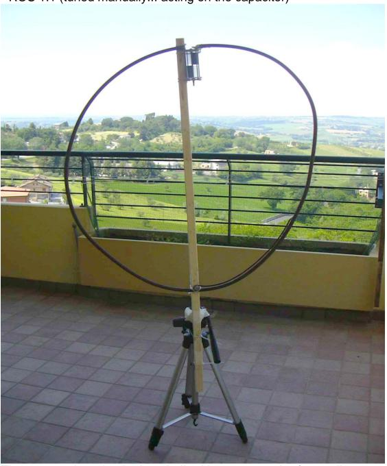
The antenna is a circular loop built with a copper tube (outer diameter 14mm, thickness 1mm).
