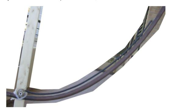
the gamma match is a simple 48cm piece of RG58/U with the inner conductor and the shield
