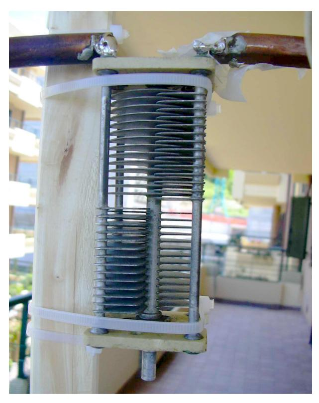
Finally, on the top in picture shown above, is welded a variable tuning capacitor, a butterfly capacitor (it's important to avoid sliding contacts in the perspective to use an ATU in the future, to avoid sparks due to the high voltage generated). Its range is [41,117]pf measured between the two external fixed plates, moving the electrically insulated rotor. Each capacitor (measured between the single plate and the rotor) is [40,190]pF. Follow that a little residual stray capacitance in the range
