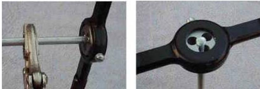
**Figure 13: Cutting the threads**
