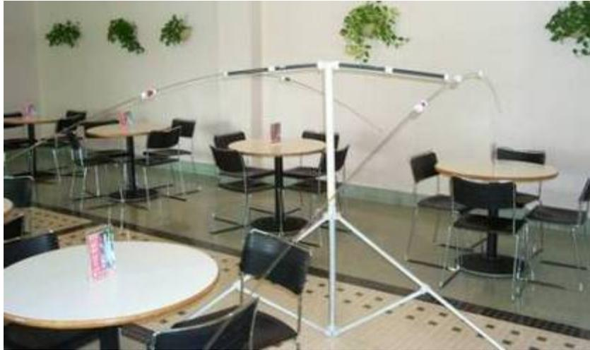
**20m beam made with PAC-12 antennas (by KA5DVS)**
