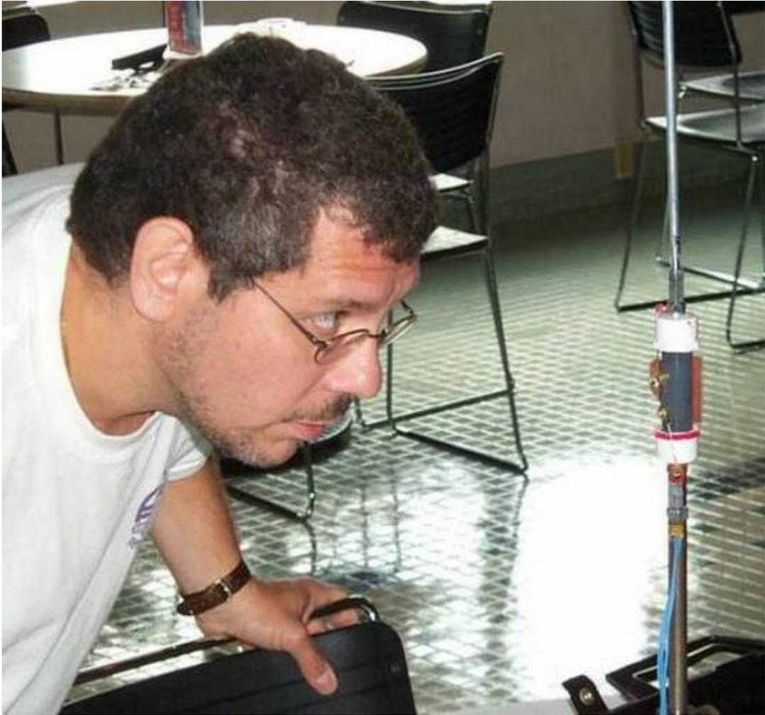
**AD2A checking out a PAC-12 feedpoint insulator made by K2MGM**
