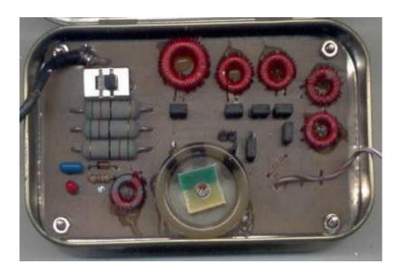
A basic resistive bridge SWR meter with LED indicator is included on the board for adjusting the tuner. The L tuner is a series L, shunt C configuration. The L consists of five toroids, with the values 8 uH, 4 uH, 2 uH, 1 uH and 0.5 uH. Shunt plugs allow shorting out each inductor, so a wide range of inductance values can be achieved, from 0.5 uH to 15.5 uH.
