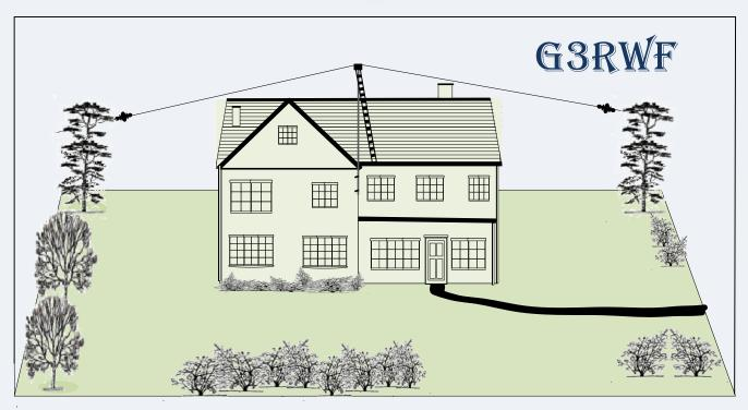
The centre of the doublet is supported by a mast on the house roof - about 55 feet up. The ends are supported by trees at about 45 feet above ground. The 60 ft of 450 ohm commercial ladder line is routed through a wall into the house to an antenna matching unit (Palstar AT1KM)
