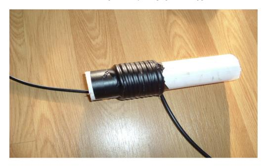
This Antenna is DC grounded by the matching transformer and a choke balun is a must to stop the feeder radiating. Here (as close to the feed point as poss) I wound 8 turns of the coax round a piece of waste water pipe.
