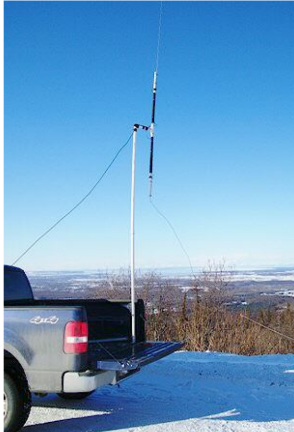
40 - 10 meter vertical dipole ready for action!
