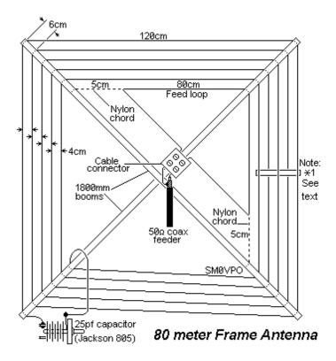
**The construction** of the antenna is shown above and is a five turn loop of one cable from 5 ampere mains cable.
