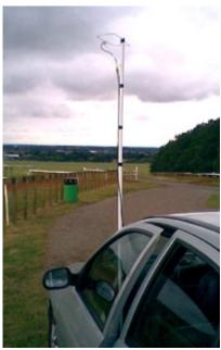
A local highspot was chosen for the contest. Highspot is a relative term as there are few real hills in this part of the UK and this "bump" behind the town of Newmarket QTH JO02DD is only around 30m ASL! Fixing the antenna to the support "mast" and trapping the mast in the car door, it was time to plug in the FT817, turn on and see what could be heard and worked.
