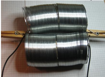
The purpose of the 80 metre slinky dipole is to allow operation on that band with a loft antenna and the design is adapted from the various offerings to be found <u>on-line</u>. In this case the slinky dipole forms part of the <u>fan dipole</u> already described.
