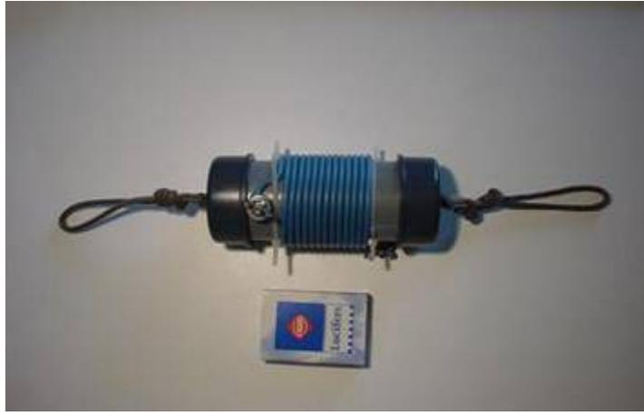
Picture 1: Trap construction with inside capacitor and 5,4  $\mu\text{H}$  inductor
