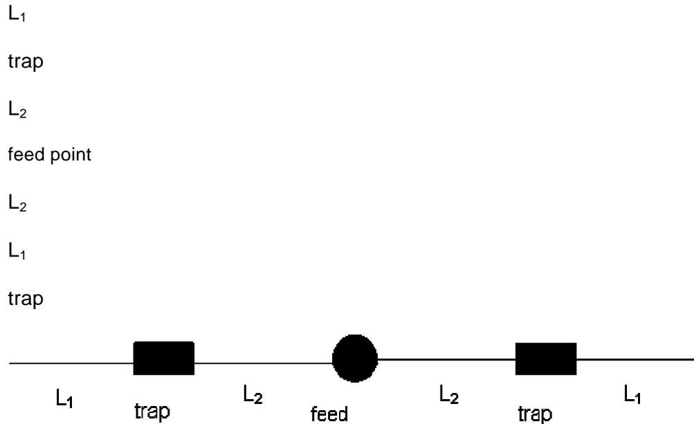
Figure 1: Trap antenna model
