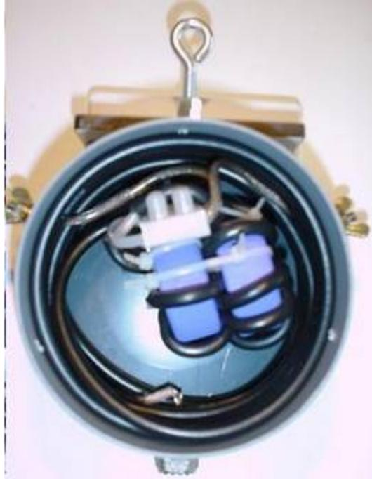
Picture 2: Impedance transformer 1 : 2.25 on two 4C65 toroides
