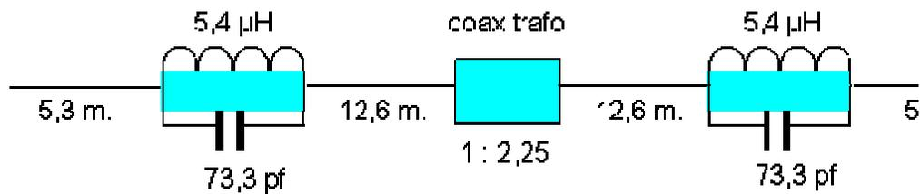
Figure 4: Antenna for most part of the five classical HF bands
