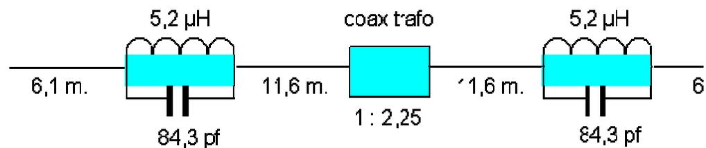
Figure 3: 4-band trap antenna
