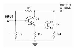
contrast, with most of these models the use of a constant-voltage DC source would cause the current to vary widely with small changes in supply voltage, temperature change, and device-to-device variations. Stable operating point needs an external series resistor between the amplifier and a DC voltage supply to approximate a constant-current source.
