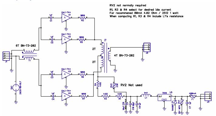
The Z10046A comprises four Mini-Circuits GaLi-74+ Monolithic Microwave Integrated Circuit (MMIC) amplifiers, U1-U4. The GaLi-74 amplifiers have 50 ohms input and output impedance and a typical gain of 25.1 dB, with OIP3 of +38 dBm and a 1 dB compression point (output) of +19 dBm. The GaLi-74's lower frequency limit is determined by the input coupling circuit, and the upper -3 dB point is 1 GHz. The noise figure is 2.7 dB.
