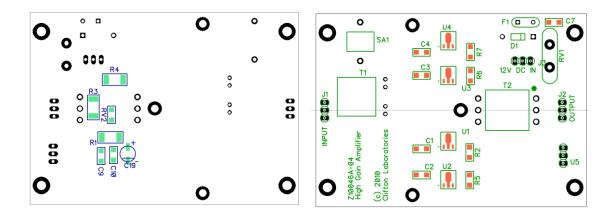
Z10046A Copper Foil Thickness. The Z10046A PCB is constructed with copper thickness three times that of a typical PCB. This is done to aid thermal tracking of U1-U4, necessary for best 2<sup>nd</sup> order intermodulation performance. From the prospective of the builder, the extra copper thickness requires a larger soldering iron and possibly a higher temperature setting than used for normal printed circuit board assembly, particularly when soldering ground pads.
