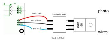
Mount U5 using 4-40 hardware (supplied with the Z10046A) and attach the 3-pin header socket to U5. It may be a tight fit to push the socket over the pins. Orient the socket as shown in the illustrations.
