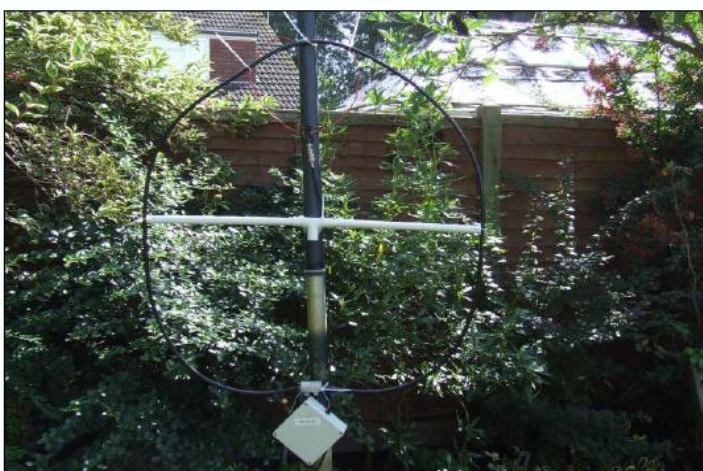
The 3m circumference RG213 loop with a remotely controlled tuning capacitor connected. ( RSARS e-Library article for more details)
