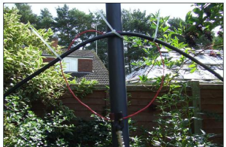
The coupling loop is 20% of the main loop's circumference to match a 50 ohms feeder. Shown here is simple wire loop made with a BNC-4mm terminals adapter- see notes further on.
