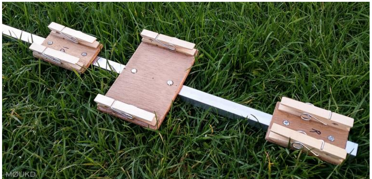
The driven element has a larger plate to accommodate the box which contains the choke and driver assembly.
