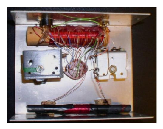
n use this Antenna Tuner works best with a Long or Random wire antenna. As little as 5 metres of copper or aluminium wire suspended and insulated at each end in a garden will make an efficient antenna. The noise will also be lower than if using a receiver indoors. In use, the receiver is tuned to a frequency, S1 is turned for strongest signal and then C1 and C2 adjusted for best reception.
