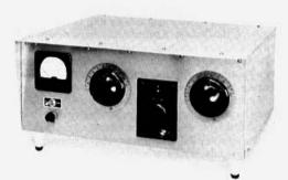
The kW version of the Ultimate Transmatch. The knobs and dial counter are standard Millen components. The front bottom of the cabinet is tilted by means of two 2-inch standoff insulators used as feet.
