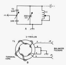
Fig. 2 — At A, details for padding a low-value variable for C1 by installing a second variable, C3, the same value as the low-power unit C2. In the case of tuning 160 meters, using an inductor of 28 uH for L1, and 250 pF per section for C1, a fixed capacitor of 100 pF can be used at C3, Centralab type 850-100N, or similar. At B, details for connecting the bifilar windings on the balun are given. The ungrounded leads a and b are connected to J3 and J4, the feed through insulator terminals.
