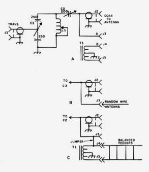
Fig. 1 - Circuit diagram of the Ultimate Transmatch.
