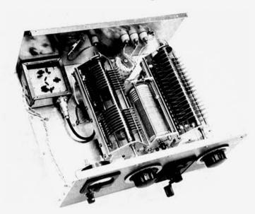
At the rear of the roller inductor is the 1-to-4 balun. The balun is set on top of a standoff insulator and is held in place with a piece of insulated board and a screw. The fixed capacitor mounted on the rear wall is the 160-meter unit. Both the variable capacitors and inductor are mounted on 1-inch high standoff insulators.
