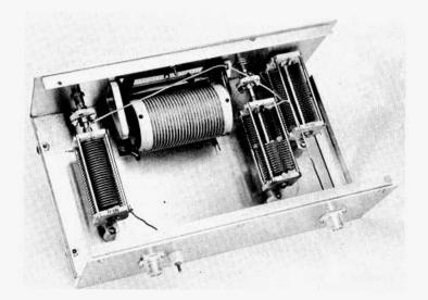
This is the low-power Transmatch. The salvaged roller inductor is mounted on the front panel, making use of the original mounting brackets.
