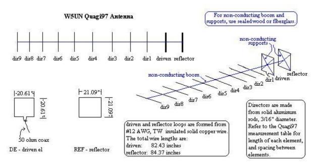
The W5UN Quagi 97 is a computer optimized quagi derived from the original W5UN Quagi of the early 1980s. The length of the 1997 model has been deliberately shortened to allow it fit on a 24 foot boom. Performance is substantially higher than that of the original antenna. It now compares favorably with yagis of the same length. The two programs used to optimize the updated antenna were AO6 and NEC 2.
