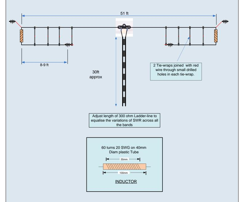
The coils require 8-9 ft of additional extension wire to tune the half-size G5RV antenna on 80m. The extension wires are folded under the main part of the antenna. The separation should be at least 6 inch (150mm). The wire spacers can be made from two plastic tie-wraps that are held together with some wire. The bottom end Insulators are not necessary, but may come with a commercial kit.
