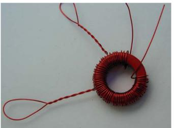
"BLOB" back and forth. The result will be a nice tin coating at the end of the wire. Check to see if the tin is all around the wire. If not, do the same procedure again. When all the ends and taps are tinned, solder L1/L2 to the 1st place, as described.
