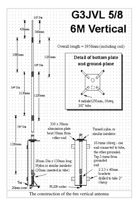
The four ground plane elements are Constructed from 1250mm long, 9.5mm (3/8") diameter aluminium tube. These are mounted to the base plate by the use of eight stainless steel machine screws. This arrangement allows easy disassembly.
