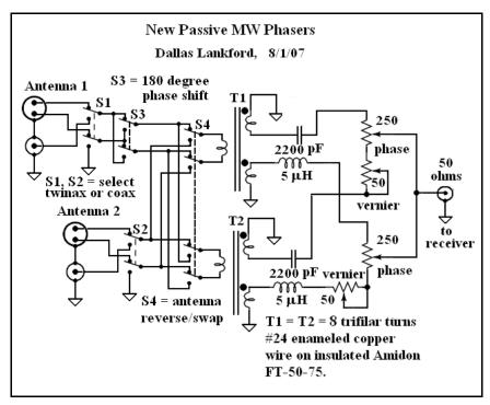
I custom built one using parts from other rotary switches. As an experiment, instead of 50 ohm pots for the vernier controls, I used two 100 ohm pots which I had on hand with fixed 100 ohm resistors in parallel with the pots. These modified 100 ohm pots are not quite as linear as 50 ohm linear pots, but they are close enough.
