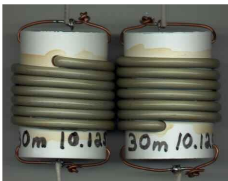
The 30 meter traps, wound on 1.25" PVC pipe couplings.
