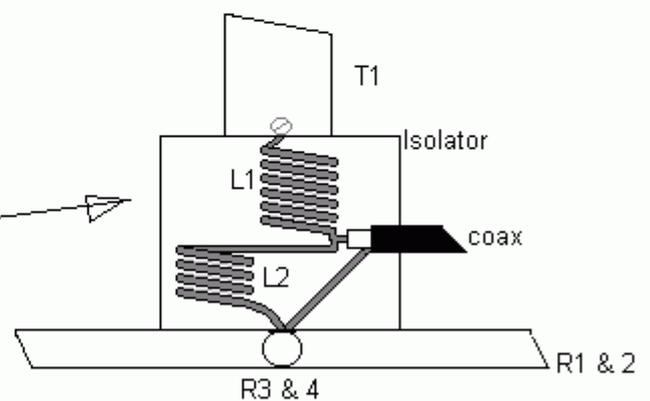
L1 = 7t 0.8mm, coil  $\varnothing$  10mm
