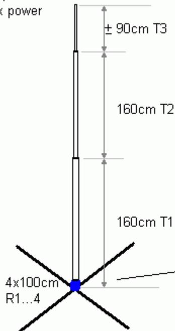
T3 = 10mm  $\varnothing$  (tune for best SWR by sliding it in or out T2)
